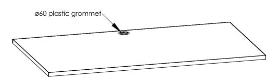
ConSet A/S SHEET 1 OF 1 DO NOT SCALE DRAWING NAME DATE UNLESS OTHERWISE SPECIFIED: DIMENSIONS ARE IN MILLIMETERS 11-10-24 DRAWN ΑL TOLERANCES: LINEAR: According to DIN 7168-m Tabletop 140-80S3 ANGULAR: CHECKED core of chipboard, density > 620kg/m3
